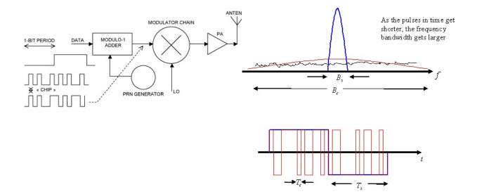
Figure 4. Spreading the spectrum in DS-CDMA
