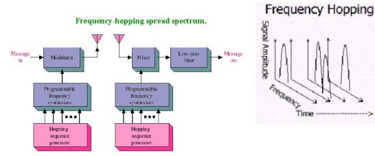
Figure 5. Spreading the spectrum in FH-CDMA
