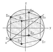
Figure 1. An example of a three dimensional constellation diagram for OFDM
